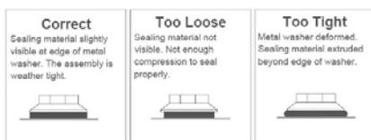
Use only fasteners with washers designed for roofing and siding applications. Fasten the outside edge first, then the center. This will prevent spreading or creeping of the panels.
