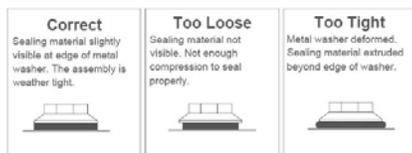
Use only fasteners with washers designed for roofing and siding applications. Fasten the outside edge first, then the center. This will prevent spreading or creeping of the panels.
